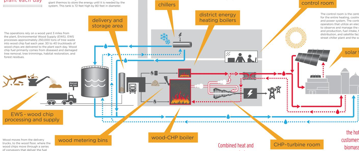
to the 5 wood metering bins. The bins control the amount of wood fuel entering the wood-CHP boiler. Careful metering of the wood into the boiler helps control the temperature, intensity, and efficiency of the fire in this boiler. The amount of wood intake will change based on the wood moisture and BTU (energy) value, as well as the boiler conditions, such as air/oxygen and natural gas input.
